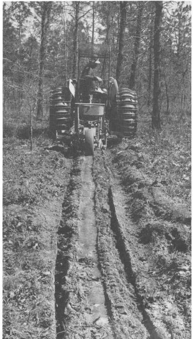
In 1958 the author invented the HC Furrow Seeder, a machine that simultaneously prepared a seedbed and planted forest seed.
