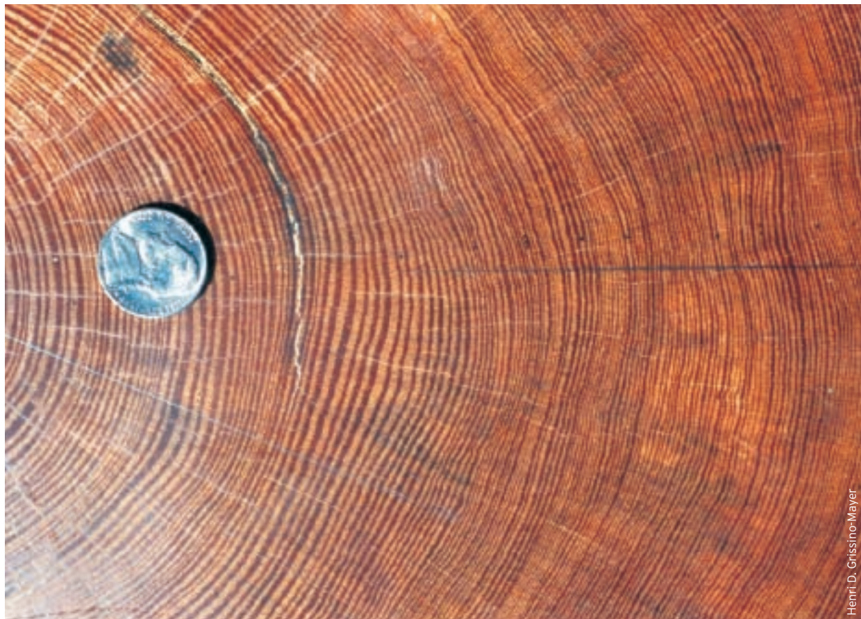
Narrow tree rings are typical for slow-growing, high density longleaf pine. This tree is from Lake Louise in southern Georgia.
