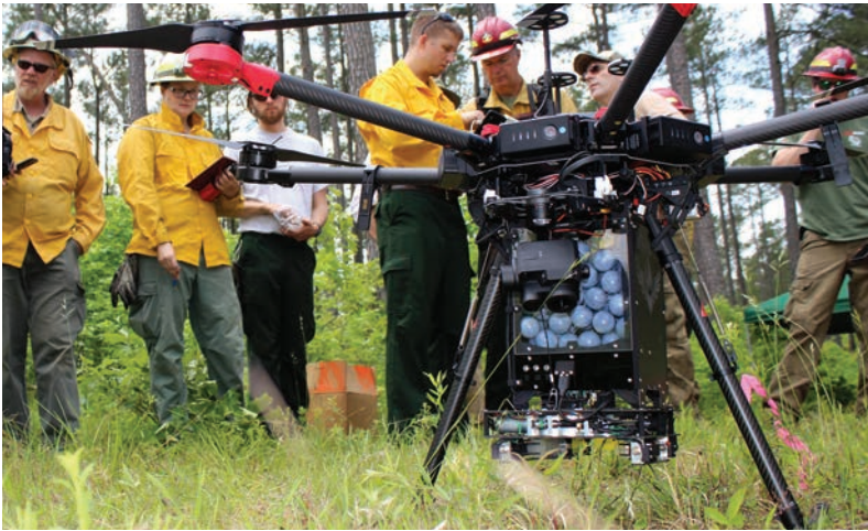
Members of the Virginia Longleaf Cooperators Group gathered at TNC's Piney Grove Preserve to observe trial flights of a drone aircraft used to assist aerial ignition operations. Photo by Daniel White.
